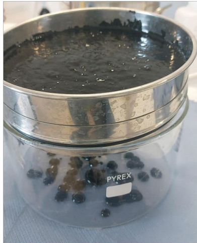
Figure 1 – Sieved post-digestate with 2 mm mesh (Source: Leitatz)
