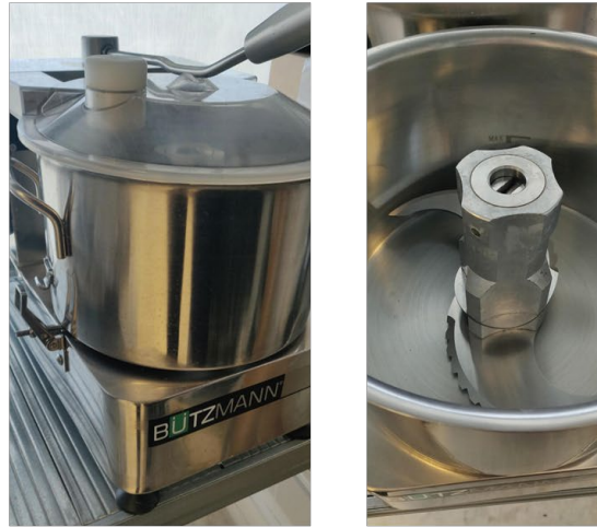
Figure 2 – Grinded post-digestate for 1 min at 1500 rpm (Source: Leitatz)
